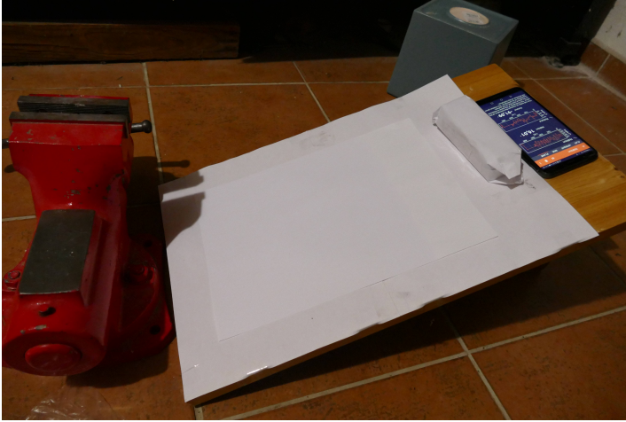
Fig. 1: Photo of experiment setup. A sheet of office paper on an inclined plane, the head of a hammer wrapped in paper, and a mobile phone. Rigid object in the back – flower pot.
